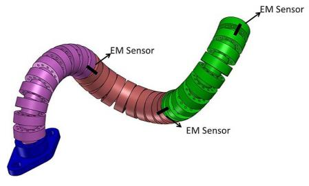
Multisection wire-driven flexible robot shown as a backbone comprising several sections. The tip position and shape information is reconstructed with two electromagnetic sensors mounted at each section's distal end (see page 4566).
